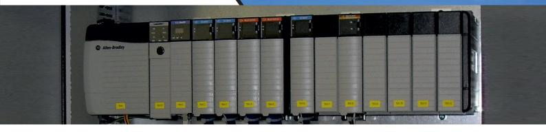
A PLC is a specialised computer intended to control machinery or electro-mechanical equipment. They also have large no of ports interacting with analog systems, sensors, switches, motors, and various other systems.
